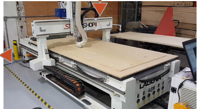
The formwork is labeled, drilled, and cut to size using in-house CNC routers. The formwork is then packed and delivered to the jobsite.
